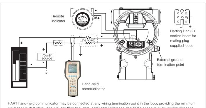
resistance is 250 ohm. If this is less than 250 ohm, additional resistance should be added to allow communications.
