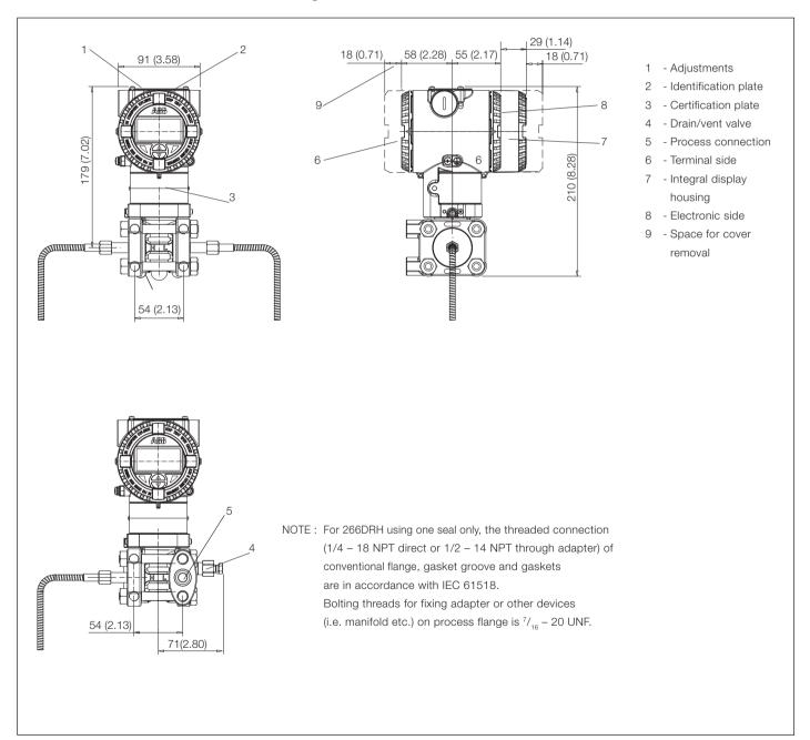
266DRH, 266PRH, 266VRH with barrel housing on bracket for vertical or horizontal 60 mm (2in) pipe
