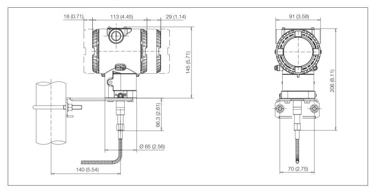
266HRH, 266NRH with DIN housing on bracket for vertical or horizontal 60 mm (2in) pipe - sensors G, H, M, P, Q, S
