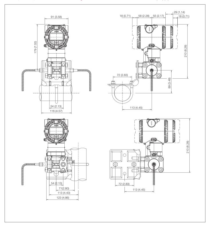
266DRH, 266PRH, 266VRH with DIN housing on bracket for vertical or horizontal 60 mm (2in) pipe
