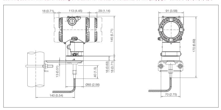
266HRH, 266NRH with barrel housing on bracket for vertical or horizontal 60 mm (2in) pipe - sensor V
